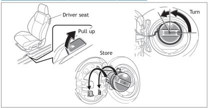
**NOTE:** Tighten cap until one click is heard. If the cap is not tightened enough, Check Engine " $\bigcup_{c \in C}$ " indicator may illuminate.
